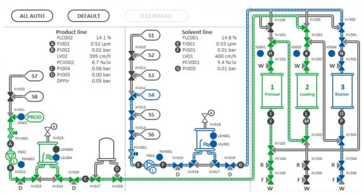
Figure 3: Common Control Platform® Software Interface V 6.0
