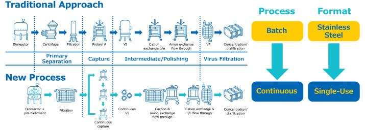
Figure 1: Continuous capture process
