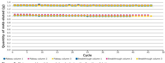
Figure 8: Plateau and breakthrough levels during the fourth validation run
