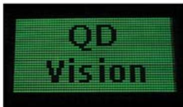
**Figure 2.** Photograph of QD Vision's prototype QD Display. The prototype is fabricated using the contact printing technique, resulting in high levels of uniformity over a 1.4" diagonal screen.
