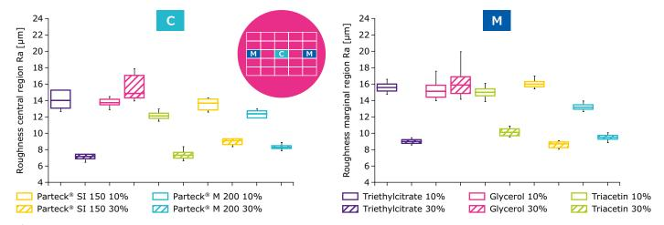
Influence of different plasticizers on the roughness of the tablet surface measured in the center (C) and margin region (M) of the tablet.
