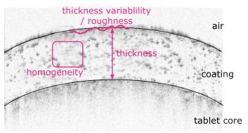
**Figure 7.**OCT enables visualization of the coating process and quality.
