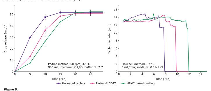
Release profiles of ascorbic acid tablets coated using Parteck® COAT, a cellulose-based polymer or without a coating.
