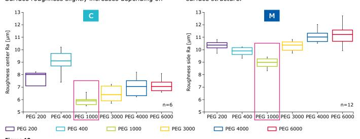
Comparison of the effect of different PEG plasticizers on tablet surface roughness.
