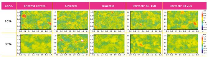
**Figure 9.**Effect of different types and concentrations of plasticizers on tablet surface roughness.
