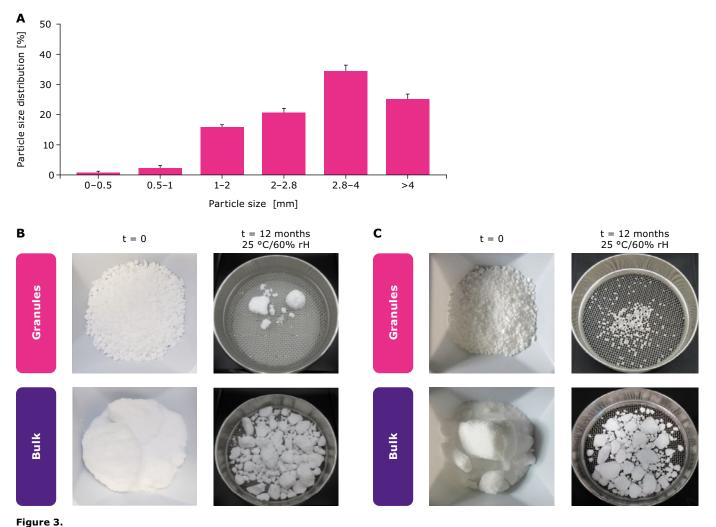
Material characteristics after dry granulation using roller compaction: A) urea particle size distribution, B) appearance of granulated urea following a 12-month stability study and C) appearance of potassium chloride following a 12-month stability study.
