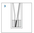
Insert the test strip in the tapered slit in the reaction vessel. The groove holds the strip in the middle of the reaction chamber (fig. 3).
