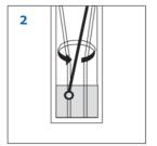
2. Suspend the bacterial mass in a reaction cuvette containing 200 µl deionized water and place the reaction vessel in the tray (fig. 2).
