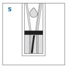
6. In order to detect indole formation, add one drop of KOVACS' reagent to the cuvette (from the dropping bottle). The appearance of a red colouration after 1–2 minutes signifies a positive reaction (fig. 5).
