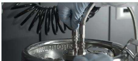
**Note:** The quick couplings on the thread adapter are of different types, in order to avoid a mix-up between gas and product connector.
