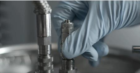
4. Remove the venting connector by pulling the knurled ring of the quick connector backwards until it is completely disconnected.
