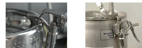
**Note:** The first few milliliters withdrawn should be disposed of in order to prevent possibly transferring production-related impurities into the solvent.
