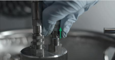
4. Use a venting connector (9.67100.1052) with the male connection (gas side, "IN") of the threaded adapter to depressurize the container completely.
