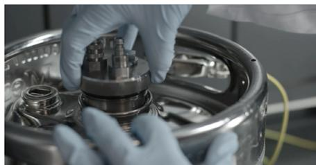
10. Keep the end of the dip tube inside the container until the remaining amount of solvent has completely dripped out of the dip tube.
