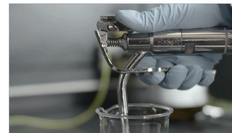
16. Hook the filling nozzle onto the head hoop of the **barrel** securely.
