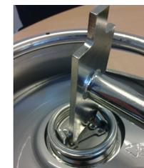
13. Disconnect the empty container from the ground. The grounding cable can be stored away in the anti-static set case (1.07070.0001) until the container is changed again.
