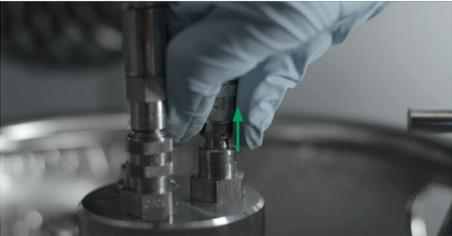
3. Use a venting connector (9.67100.1052) with the male connection (gas side, "IN") of the threaded adapter to depressurize the container completely. **Make sure that the gas emitted is not contacting the user but is deflected away to the air extraction device.**
