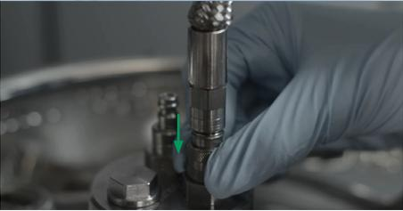
5. Disconnect the product hose (incl. filling nozzle) by pushing the knurled ring of the quick connector on top of the treaded adapter downwards until it is completely disconnected from the threaded adapter.
