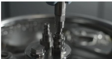
10. Hook the filling nozzle onto the head hoop of the **barrel** securely.
