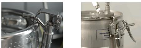
11. Connect the gas feeding tube with its rapid-action connector to the male connector marked "IN" on the threaded adapter.
