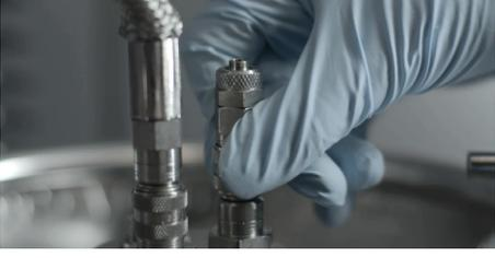
5. Remove the venting connector by pulling the knurled ring of the quick connector backwards until it is completely disconnected.
