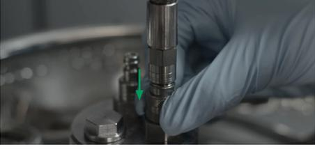
6. Disconnect the product hose (incl. filling nozzle) by pushing the knurled ring of the quick connector on top of the treaded adapter downwards until it is completely disconnected from the threaded adapter.
