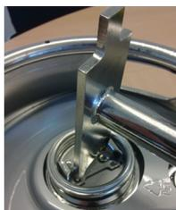
9. Unscrew the threaded adapter with the dip tube from the empty container.
