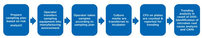
Figure 1: Process steps for Environmental Monitoring (classical microbiological part)
