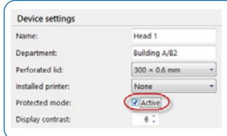
Protected mode: Checkbox <<Active>> Switches the protected mode for the instrument on.
