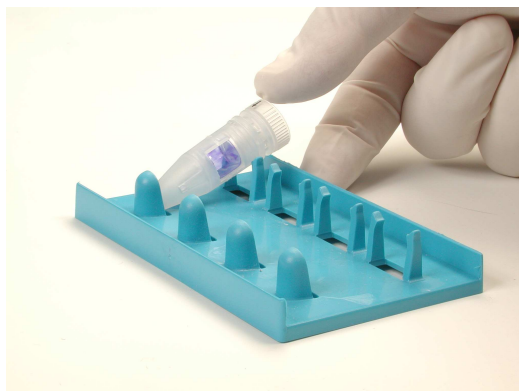
Figure 3. Insertion of D-Tube™ Dialyzer in Supporting Tray Midi showing correct orientation of membranes, which must be perpendicular to the electric field.
