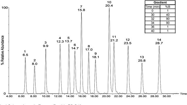
Dual Column Ascentis Express Peptide ES C18 (1 mm I.D.  $\times$  15 cm length, 2.7  $\mu$ m particles, 40 °C) at 90  $\mu$ L/min Solvent A: 0.1% formic acid Solvent B: Acetonitrile with 0.1% formic acid
